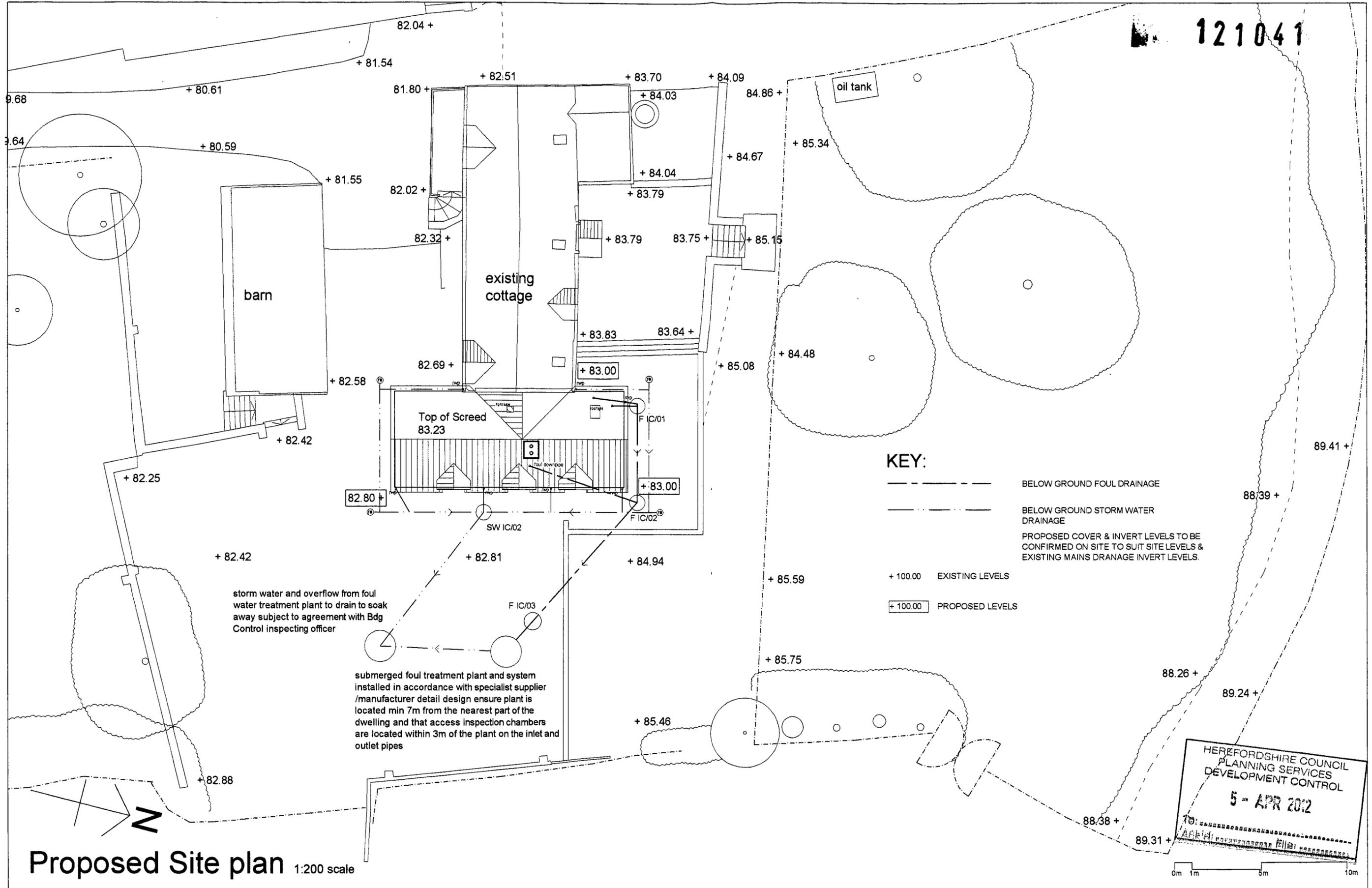
Proposed Site plan 1:200 scale
